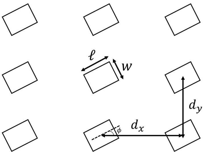
$$(a, \ell, w, d_x, d_y, \phi) = \\ (5.627 \text{ um}, 58.59 \text{ um}, 50.78 \text{ um}, 249.3 \text{ um}, 198.2 \text{ um}, 27 \text{ degree})$$
